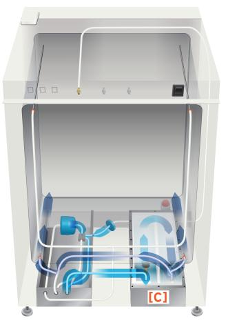
The In-Vitrocell direct heat incubator routes fresh air and gas through disk filters on the front **[A]** and constantly recirculates existing chamber air through a separate bay located under the chamber **[B]** where a HEPA filter cleans it, and gas sensors measure its  $CO_2$  and  $O_2$  levels. The air is returned to the chamber after passing through a humidity reservoir if more humidity is needed **[C]**.\*
