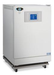
Direct-heat CO<sub>2</sub> incubators, such as **NuAire's In-VitroCell series**, offer two types of heat decontamination cycle. A 95°C humidified cycle or 145°C dry cycle can decontaminate the interior of the incubator.
