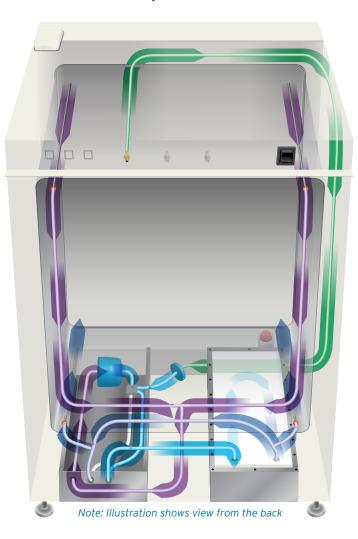
Air is passed through a reservoir if moisture is needed\*
