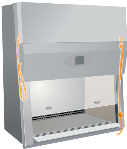
Remove user-accessible wiring for disposal.
