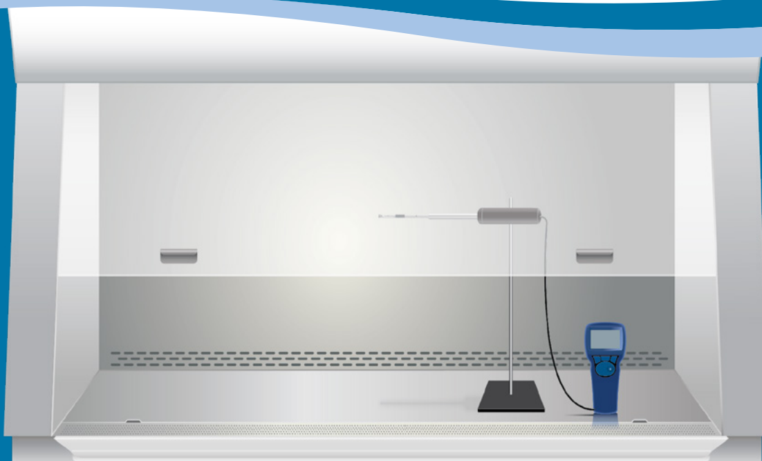
Airflow probes are used to calculate the downflow velocity of biosafety cabinets.
